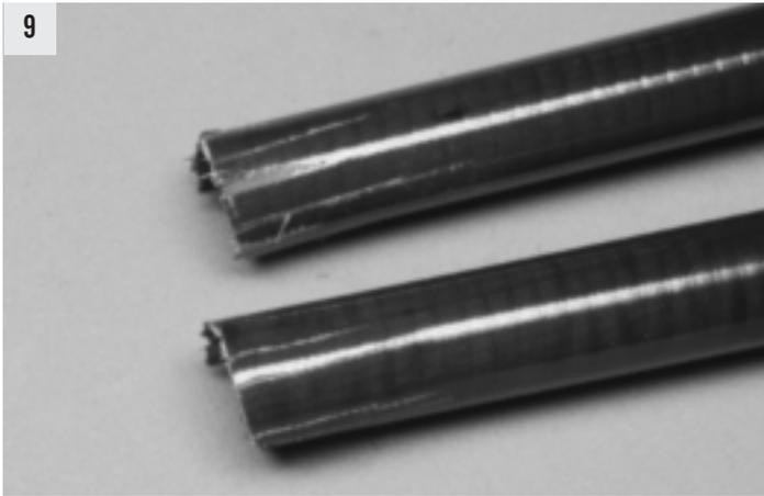
you no longer have a tube and a catastrophic failure is the result. Load limit failures are easy to spot. This type of break will always take place in the bottom half of the rod, usually just forward of the handle or the fisherman's furthest point of effort (the rod hand). The break will be slightly irregular with jagged edges and short lengthwise splits and tears (9). Looking at the inside of an overload failure you'll note great distress in the walls of the blank both inside and out (10).
